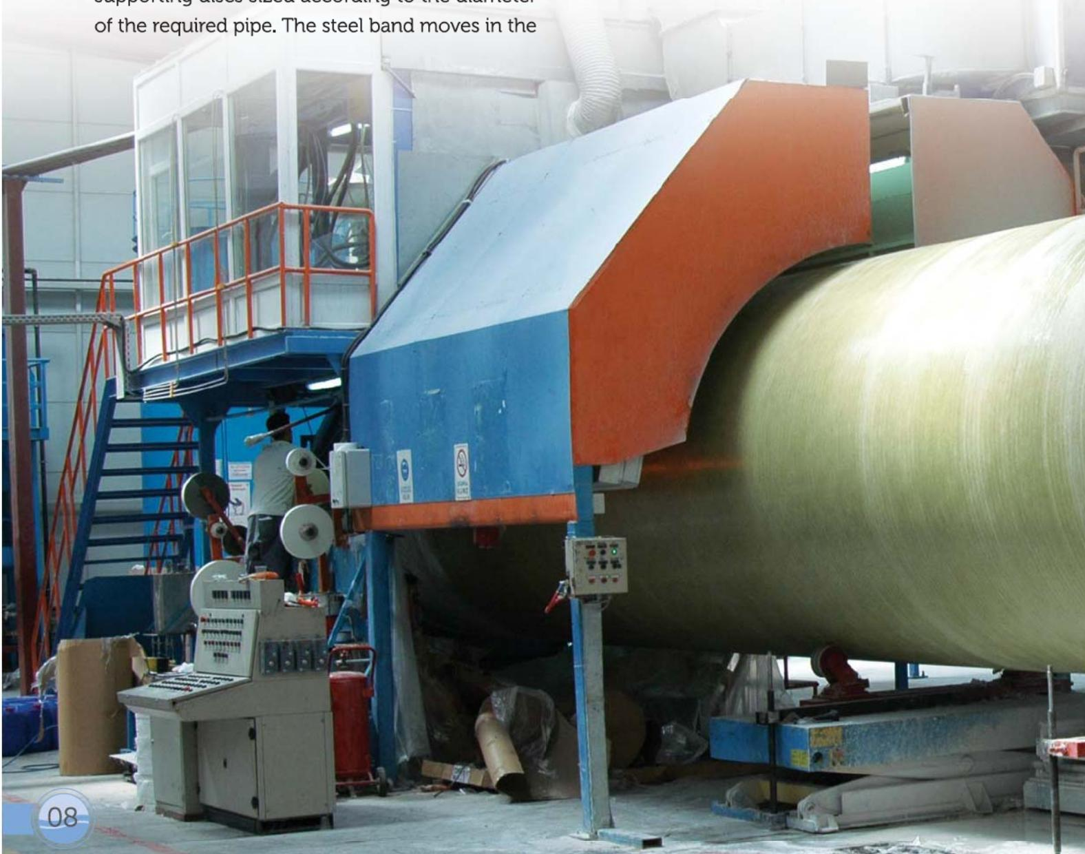
Glass roving together with chopped glass, sand aggregate, polyester resin are applied simultaneously on the proper mandrel positions according to GRP pipe design specifications. At the end, a layer of surfacing mat is applied.
