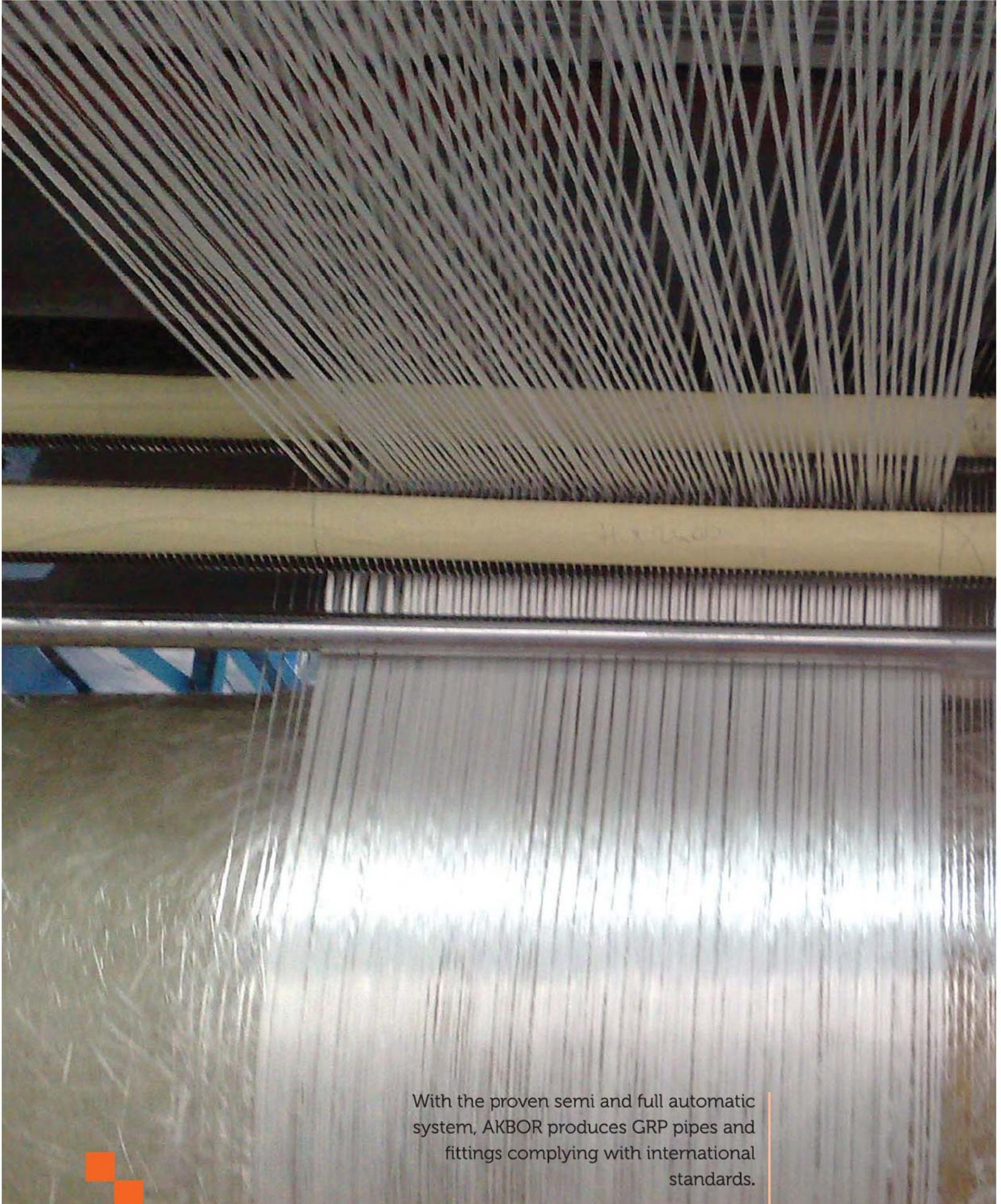
With the proven semi and full automatic system, AKBOR produces GRP pipes and fittings complying with international standards.
